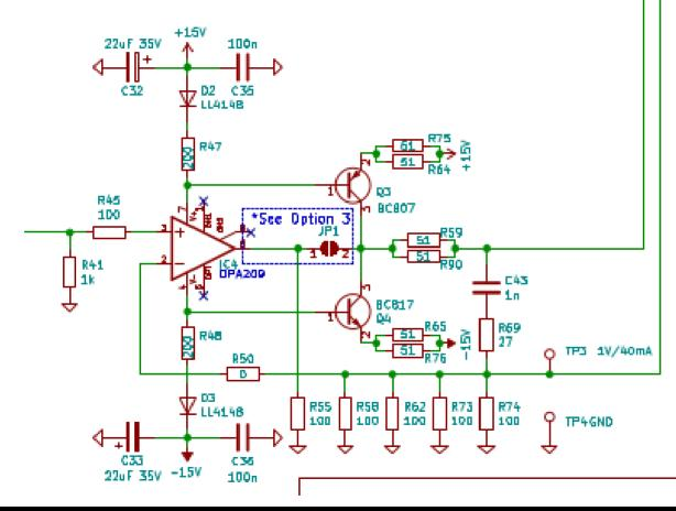
Option 3: Low FM Current Solder JP1 connection Bridge D2 and D3 R47, R48 = D Q3, Q4, R55 = DNP R64, R65, R75, R76 = DNP R59, R9D = 470
