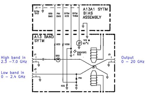
HP 5086-7414 Coil: 50 ohm (15 mA/GHz) Heater: 295 ohm to GND
