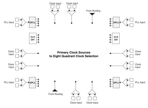
$Note: This \ diagram \ shows \ sources \ for \ the \ XP2-17 \ device. \ Smaller \ Lattice XP2 \ devices \ have \ two \ GPLLs.$
