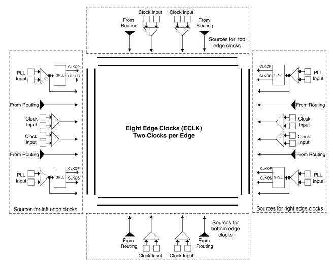
Note: This diagram shows sources for the XP2-17 device. Smaller LatticeXP2 devices have two GPLLs.
