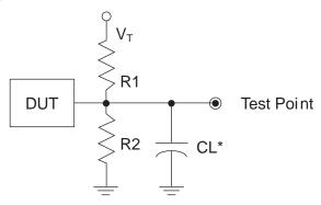
\*CL Includes Test Fixture and Probe Capacitance
